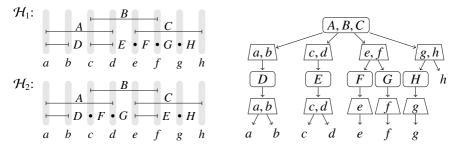
Figure 3: An interval hypergraph  $\mathcal{H}_1$  and its overlap component tree. In the tree, the node of an <u>overlap component</u> O is given by listing the hyperedges in O; a <u>slot</u> node  $S_O$  is given by listing the vertices contained in S (we omit the reference to O as it is understood from the tree structure). The hypergraph  $\mathcal{H}_2$  is not isomorphic to  $\mathcal{H}_1$ ; yet both have isomorphic overlap component trees.
